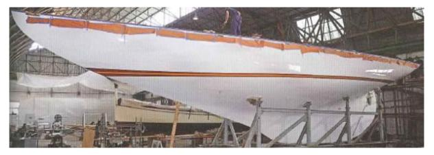
In particular, the unit is characterized by a high ratio length to width, as well as by a high construction height, features that provide high hydrodynamic performance to the front of a lower stability, which however can be restored by the high ballasting of drift (by lead).
