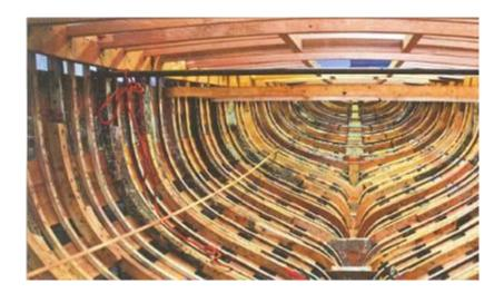
*Plating* used to waterproof the ship's resistant body (represented by the reinforcements) as well as the transmission of local loads, is made of **mahogany**;
