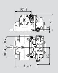
Control valve, fixed setting and hydraulic inch valve built-on, DA4/DA8
