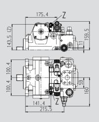
Control valve, fixed setting and connections for master controller, DA7
