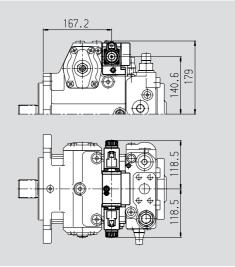
Hydraulic control, speed related, DA Control valve, fixed setting, DA2
