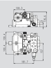
Control valve, fixed setting and hydraulic inch valve built-on, DA4/DA8
