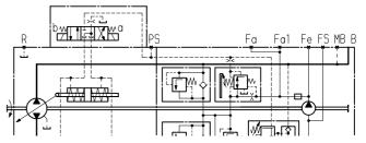
Hydraulic control, speed related, DA control valve, fixed setting, with hydraulic inch valve, DA1D4/DA2D4
