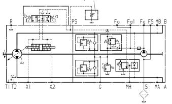
Hydraulic control, speed related, DA with separately installed hydraulic inch valve
