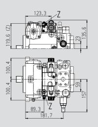
Control valve, fixed setting and connections for master controller, DA7
