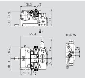
Control valve, fixed setting and connections for master controller, DA7
