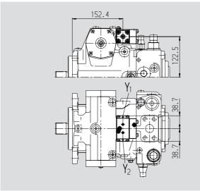
Electrical two-position control, with switching solenoid, EZ
