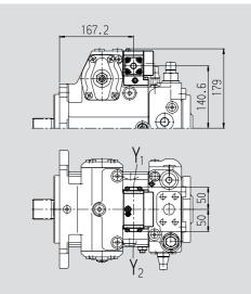
Electrical two-position control, with switching solenoid, EZ
