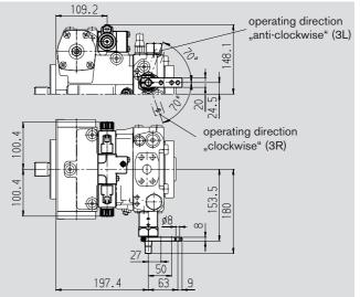
Control valve, mechanically adjustable with lever and hydraulic inch valve built-on, DA5/DA9
