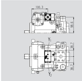
Electrical two-position control, with switching solenoid, EZ
