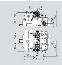
Control valve, fixed setting and connections for master controller, DA7
