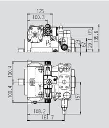
Control valve, mechanically adjustable with lever, DA3
