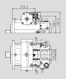
Electrical two-position control, with switching solenoid, EZ
