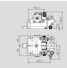
Control valve, fixed setting and hydraulic inch valve built-on, DA4/DA8
