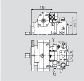
Electrical two-position control, with switching solenoid, EZ
