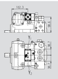
Electrical two-position control, with switching solenoid, EZ
