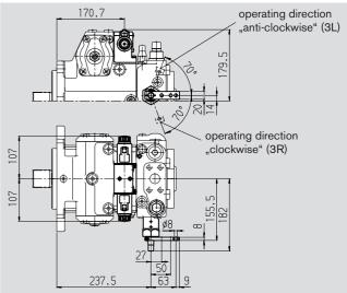
Control valve, mechanically adjustable with lever and hydraulic inch valve built-on, DA5/DA9
