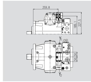
Electrical two-position control, with switching solenoid, EZ
