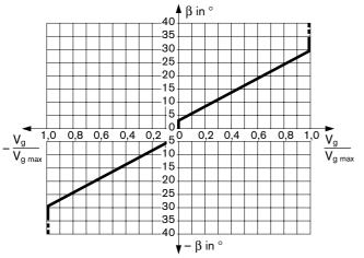
Swivel angle b at the control lever for swiveling outwards:
