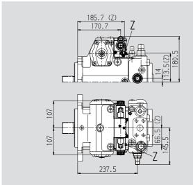
Control valve, fixed setting and connections for master controller, DA7
