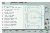
iTNC 530 HSCI is adapted not only for programs from CAD/CAM software; it also offers a number of options directly, in workshop programming. Special dialogue language with a high number of integrated cycles enables quick and productive programming of contours, drilling, etc., including programming in inclined planes.
