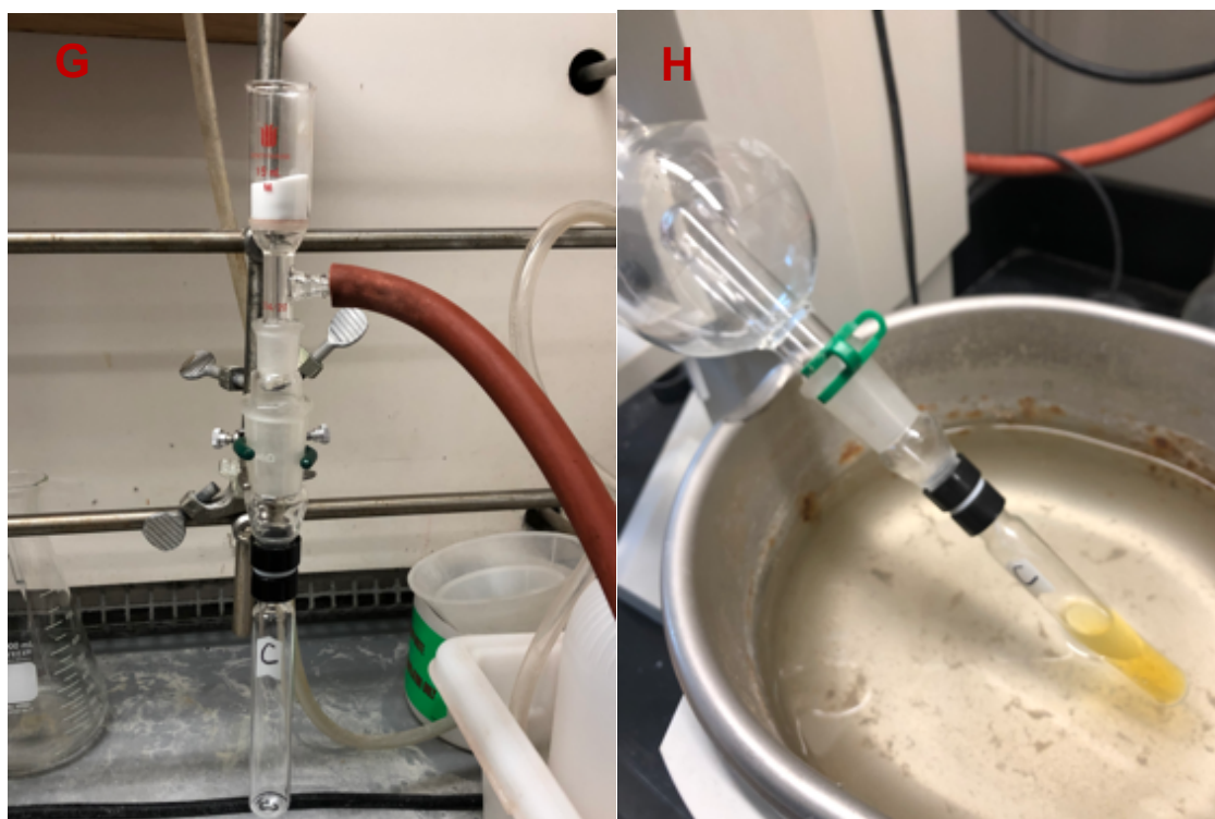
Figure S12: G. Setup for the filtration of the crude reaction mixture into reaction tube "C". H. Concentration of volatiles in vacuo by rotary evaporation.
