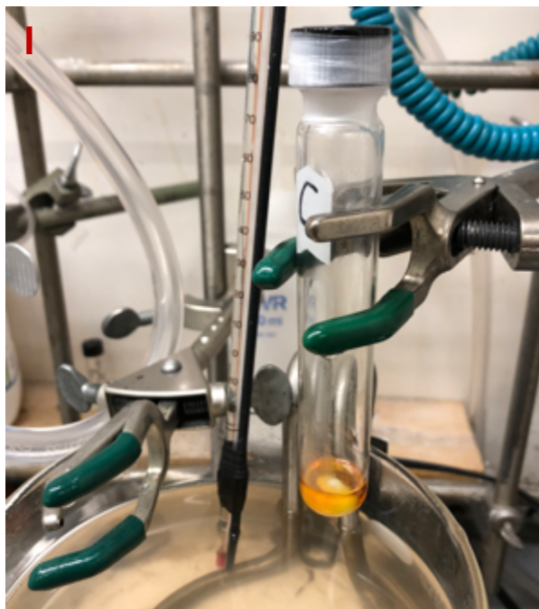
Figure SI2 I. Appearance of reaction mixture in tube “C” following the addition of toluene and alkyne, but prior to heating in a 110 °C oil bath.
