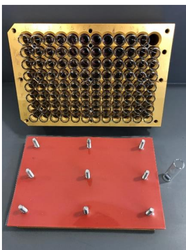
Figure S1. Representative image of a reaction block, reaction vessels, stir bar, PFA sheet, and rubber mat used in high throughput experimentation.
