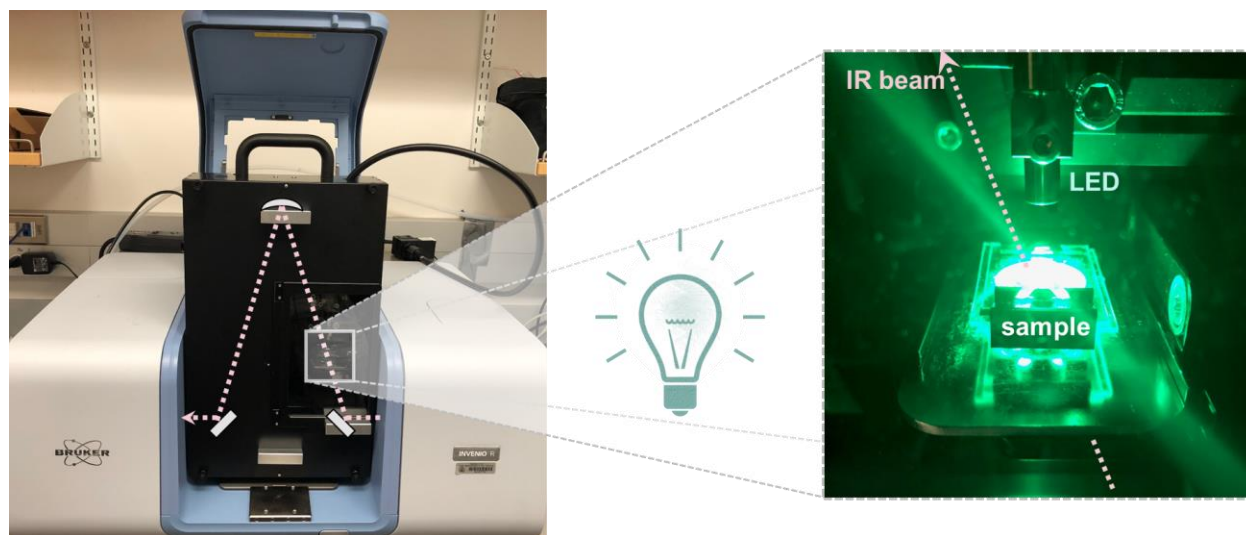
Figure S20. FTIR setup with horizontal transmission accessory for real time monitoring of photopolymerization.
