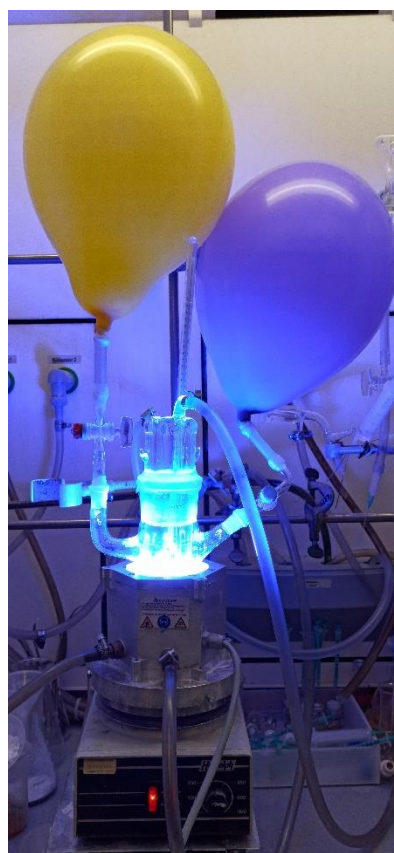
Fig. S2: Custom-built glass reactor for upscaling of the photocatalytic ammoxidation reaction.
