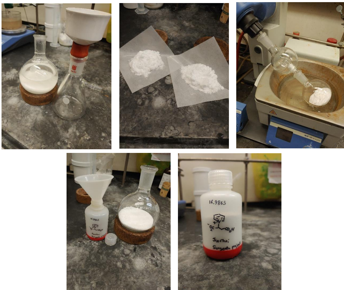
Fig. S8. Work-up procedure for 1 st step of feedstock synthesis. Precipitated solid was obtained by filtering using Büchner funnel, washed EtOAc, MeOH (upper left, center). The resulting solid was dried by rotary evaporator and high vac. (upper right), The pyridinium 9 was stored in 100 mL Nalgene bottle, stable in ambient temperature (bottom).
