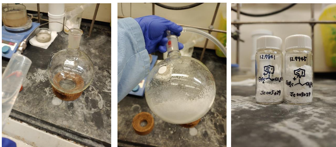
Fig. S14. Resulting pyridine feedstock. The resulting liquid after work-up was added anhydrous \text{Et}_2\text{O} for removing the residual solvent (left), dried product as a white solid (center), The resulting feedstock 6a was stored in 20 mL vial, stable in ambient temperature (right).
