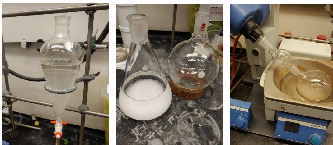
Fig. S13. Work-up procedure for to 2 nd step of feedstock synthesis (continued). diluted with \text{CH}_2\text{Cl}_2 and \text{H}_2\text{O} (left), extracted with \text{CH}_2\text{Cl}_2 , dried by \text{Na}_2\text{SO}_4 (center), filtered, evaporated residual solvent by rotatory evaporator (right).
