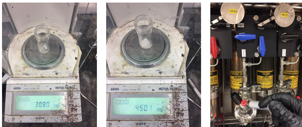
Left: \text{Bu}_4\text{NClO}_4 (308 mg, 0.9 mmol). Center: 3 Å molecular sieves (450 mg). Right: \text{CH}_2\text{Cl}_2 (9 mL)
