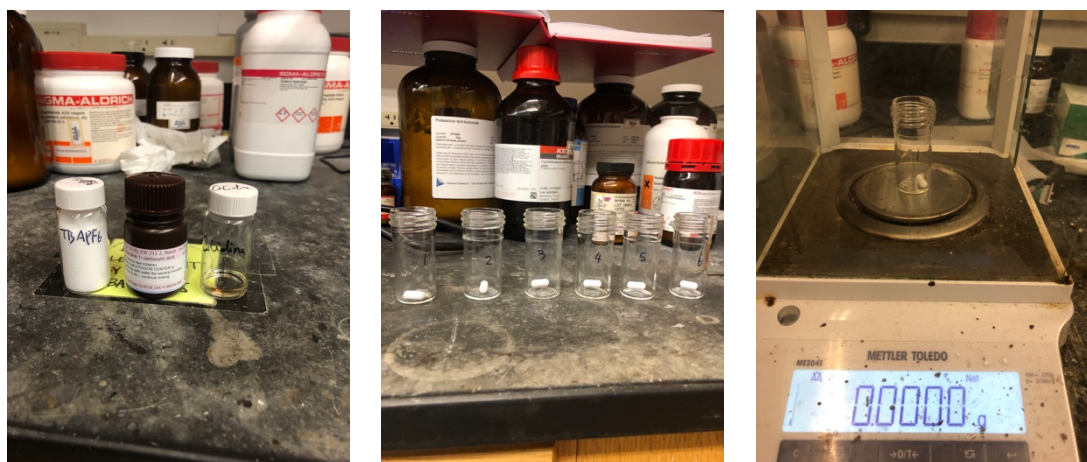
Left: reagents for hydroxylation reaction. Center: ElectraSyn vials (25 mL). Right: Tare of the vial.
