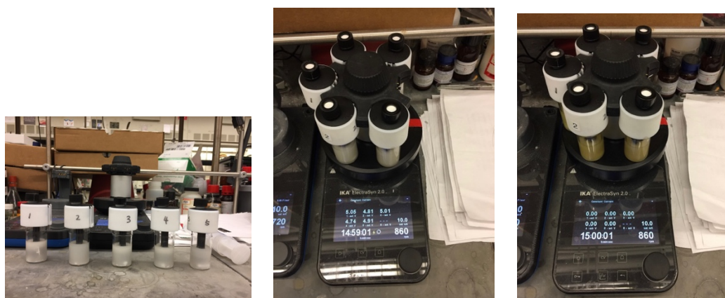
Left: after adding \text{CH}_2\text{Cl}_2 and equipped with graphite electrodes for 5 reactions. Center: start the reaction on the ElectraSyn device (after 1 min). Right: reaction completed (15h).
