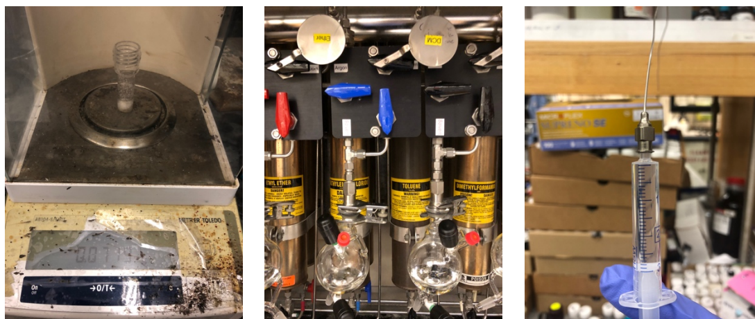
Left: 2,4,6-collidine (72 mg). Center: \text{CH}_2\text{Cl}_2 from solvent system. Right: \text{CH}_2\text{Cl}_2 (3 mL).
