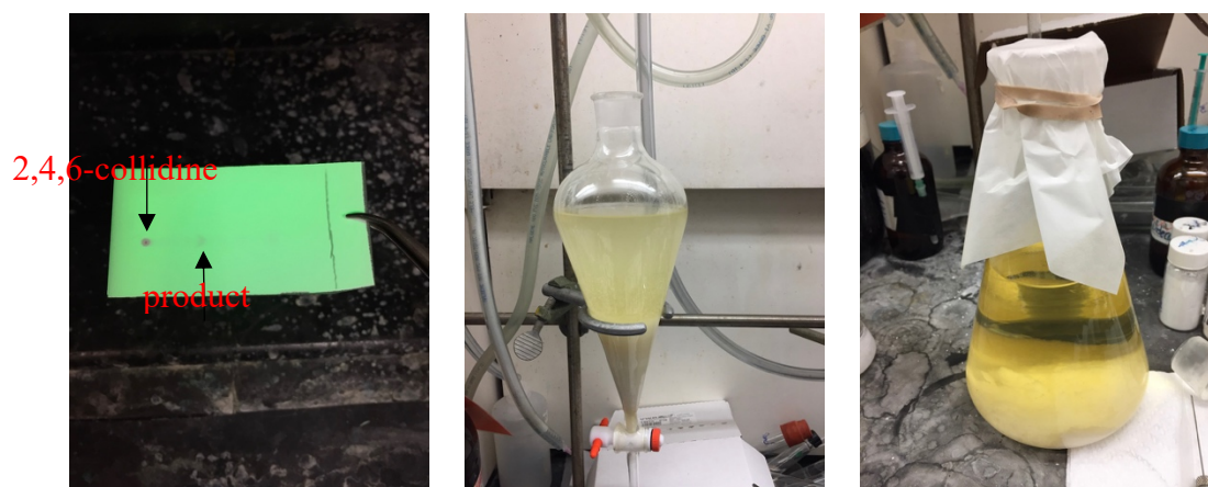
Left: crude TLC (Hexanes: \text{Et}_2\text{O} =30:1). Center: the suspension of 5 reactions was diluted with \text{Et}_2\text{O} and washed with 1 N HCl. Right: dried over \text{Na}_2\text{SO}_4 .
