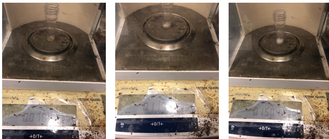
Left: \text{AgPF}_6 (76 mg). Center: n\text{Bu}_4\text{NPF}_6 (116 mg). Right: 3 Å MS (150 mg).
