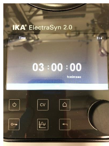
LEFT. Select “No” for using a reference electrode. MIDDLE. Select “Time” to control the reaction duration. RIGHT. Input “3 h: 00 m: 00s” as the reaction time.
