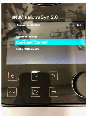
LEFT. On the ElectraSyn, select “New Experiments”. MIDDLE. Select “Constant Current”. RIGHT. Input “10.0 mA” as the reaction current.
