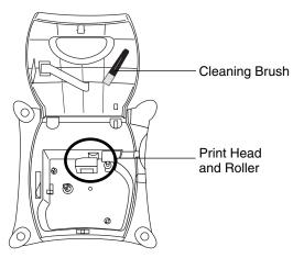
2 Gently brush the print head to remove any dust or particles.
