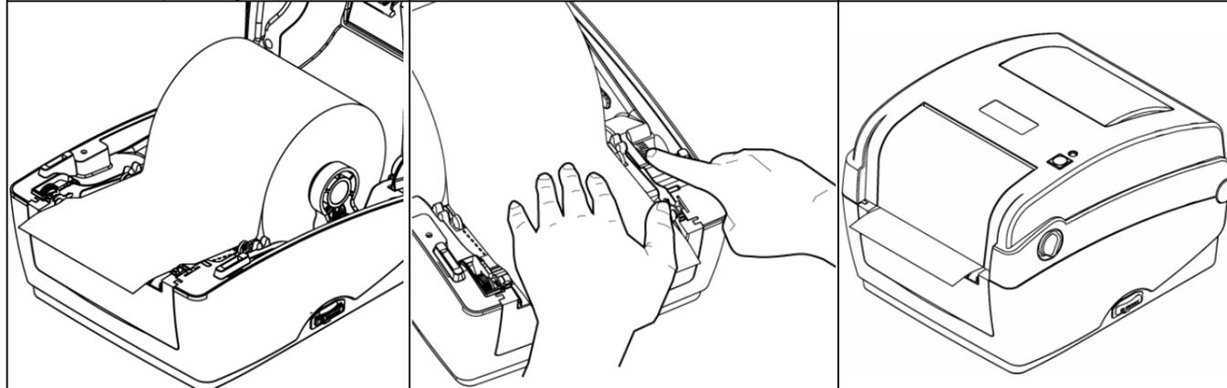
(4) Place the paper, printing side face up, through the media sensor and place the label leading edge onto the platen roller.
