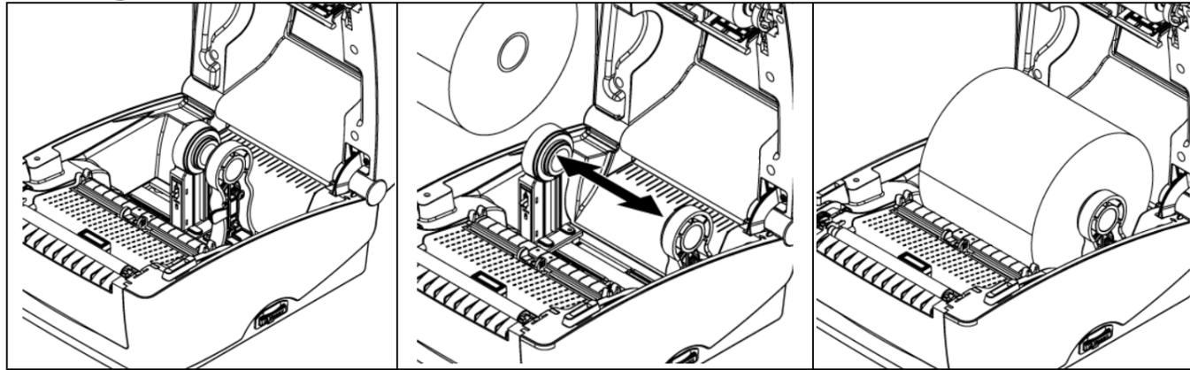
(1) Open the printer top cover by pulling the green tabs located on each side towards the front of the printer, then lift the top cover to the maximum open angle.
