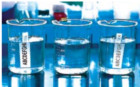
Water and chemical resistant: glass plates with laminated labels attached were immersed in water and various chemicals for two hours. The text was unaffected
