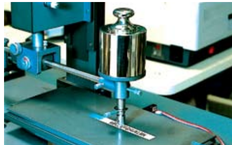
Abrasion resistant: after a 1kg sanding device was passed over the laminated labels 50 times, the text was unaffected
