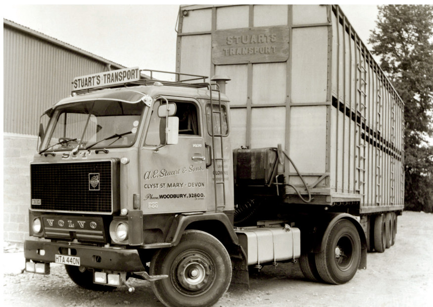
AE Stuart & Sons would operate seven Volvo F88 tractors, including this high-spec 290hp model
