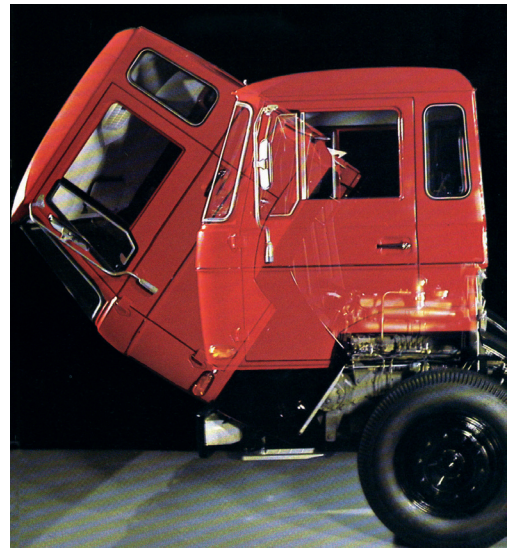
Evolving design: the 1969 DAF 218 featured a tilting cab
