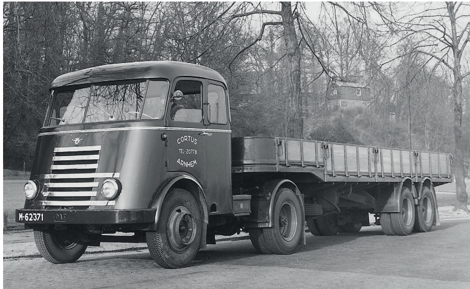
Outsourcing: early DAF trucks were driven to a local bodybuilder to have their cabs fitted
