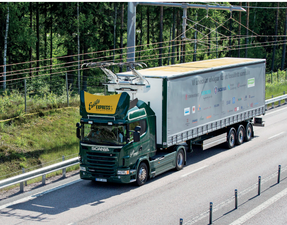
Along the right lines: electric road hybrid truck, Scania G 360 4x2 (hybrid truck with Siemens pantograph on the roof)
