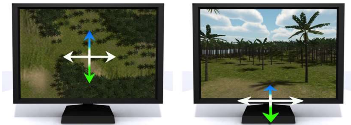
Figure 5-12. The origin of Unity navigation terminology. Left: The overhead view of a world where Vertical (on the monitor) moves you forward through the scene. Right: The directions tilted down to use in a 3D world
