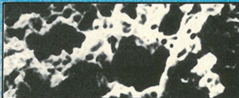
Typical conventional antifouling containing soluble rosin binder. Note skeleton layer left by dissolved rosin (reduced efficiency).
