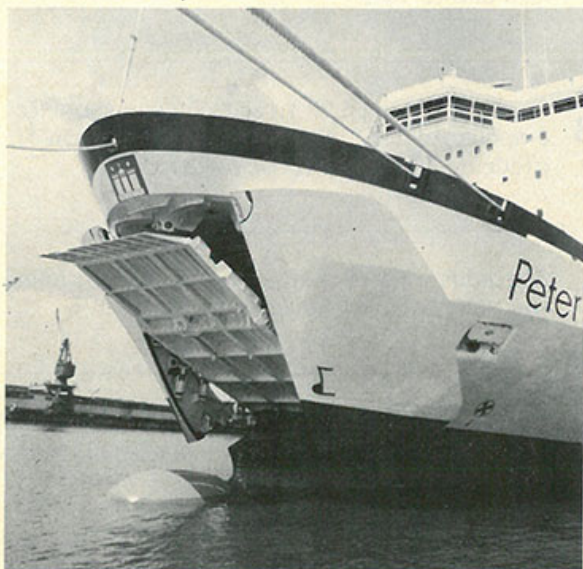
For the jumbo-ferry »Peter Pan« built at Seebeckwerft AG, the bow ramp and the drive for the double panel side swinging door were delivered by MACOR Marine Systems International.
