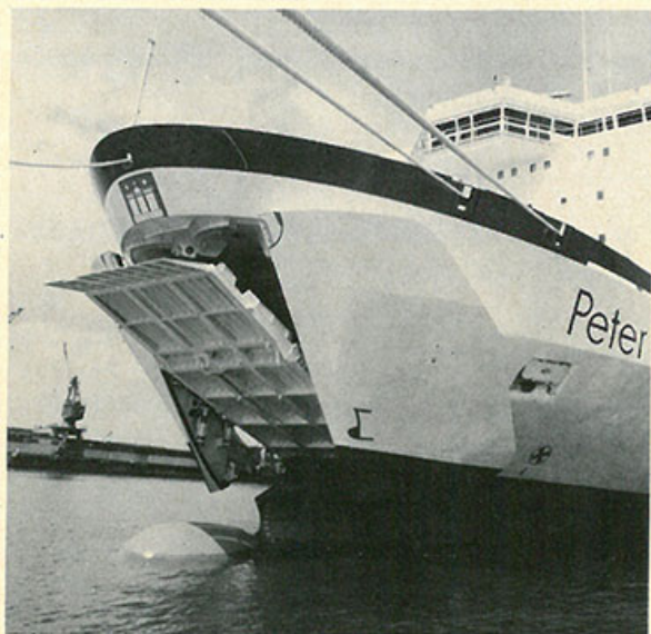
For the jumbo-ferry «Peter Pan» built at Seebeckwerft AG, the bow ramp and the drive for the double panel side swinging door were delivered by MACOR Marine Systems International.
