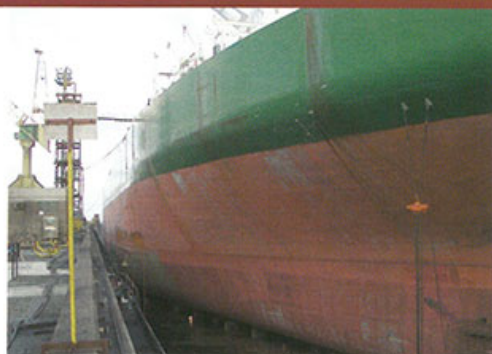
M/V Ramlah pictured during washing in drydock, Dubai, after 61 months in-service.
