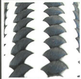
12 - strand dyneema core + protection jacket
