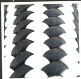
12 - strand dyneema core + protection jacket
