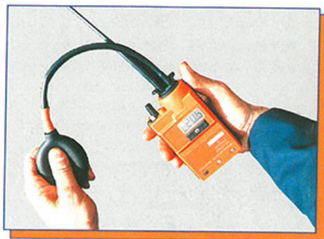
Aspirator sampling prior to confined space entry
