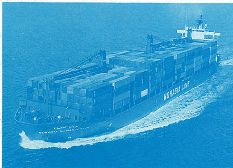
Containership powered by Sulzer 6RTA62 diesel engine.
