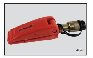
The JS4 hydraulic spreader is the ideal solution for spreading, wedging and prising operations in a wide variety of industrial applications. The compact, low weight, spring assisted return design enables the tool to fit into a gap of 9.7mm and offers a maximum spread of 94mm. Manufactured from high strength steel, with a maximum pressure of 700 Bar, the JS4 is supplied fitted with a quick connect female half coupler.
