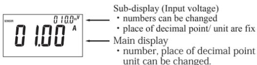
Press the LIGHT key to change displays in following sequence.
