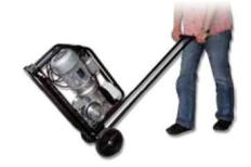
The Pulling Guide is suitable for the Katimex KSW-E series. It is a support tool for cable pulling. With it a form-fitting connection of the winch and the cable outlet is possible.
