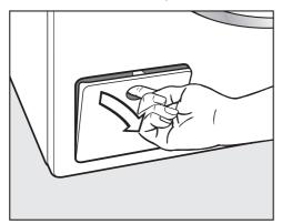
■ Open the drain pump access panel.
