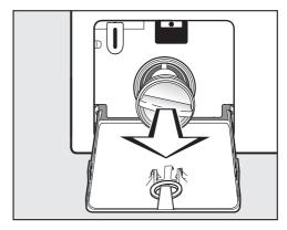
■ Remove the drain filter completely.
