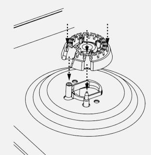
When fitting the burner head, make sure that the notch lines up with the hole in the base.
