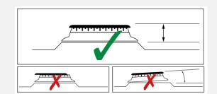
Check that the burner head is level and the cap is fitted centrally on the burner head.
