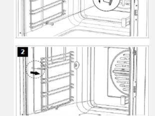
Remove holding screws as per diagrams
