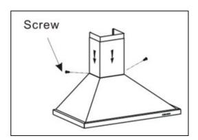
◆ Sliding the chimney to adjust the chimney height. When the height you required is reached, then fix 2 pcs of 4x8mm screws onto the hole fixing with plate I as showed in below pictures.
