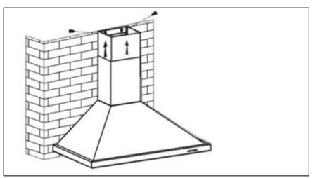
Fix the lower chimney with 2 pcs of 4x8mm screws.
