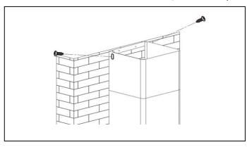
Remove all blue protective film on chimney and cooker hood, the installation is now finished.
