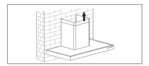
◆ Sliding the chimney to adjust the chimney height. When the height you required is reached, then hang the fixing hole to the fixing screws as showed in below pictures
