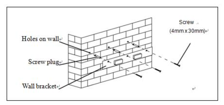
1. Offer up the cooker hood and hang onto the wall bracket hook.
