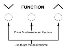
The **FUNCTION** button in the centre is used for setting the minute minder
