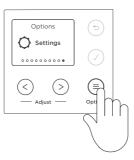
Press OPTIONS ≡, scroll to SETTINGS using the ADJUST < > buttons, press ✓ to confirm.
