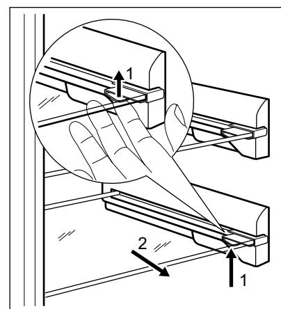
The glass shelves equipped with expander rollers are secured with locking pins.
