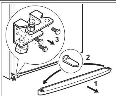
**!** To carry out the following operations, we suggest that this be made with another person that will keep a firm hold on the doors of the appliance during the operations.
