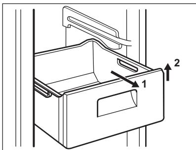
Some of the freezing baskets have a limit stop to prevent their accidental removal or falling out. At the time of its removal from the freezer, pull the basket towards yourself and, upon reaching the end point, remove the basket by tilting its front upwards.
