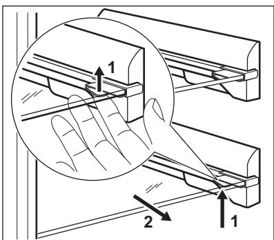
The appliance is equipped with shelf stops to secure the shelves. The shelves must be lifted up (1) on each side and then pulled outwards (2). The glass shelves equipped with expander rollers are secured with locking pins.
