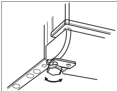
Accurate levelling prevents the vibration and noise of the appliance during operation. To adjust the height of the appliance loosen or tighten the two adjustable front feet.
