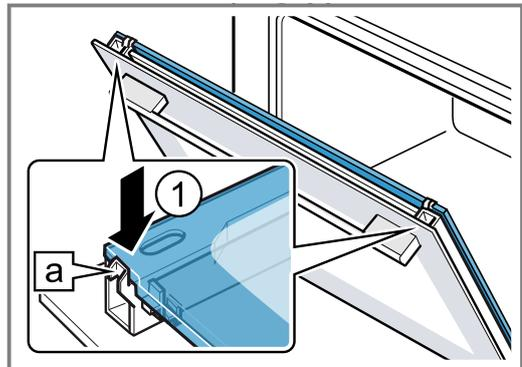
8. Put the door cover into position ① and push down on it until you hear it click into place.
