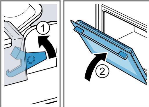
4. Push on the left- and right-hand side of the door cover from the outside ① until it is released.
