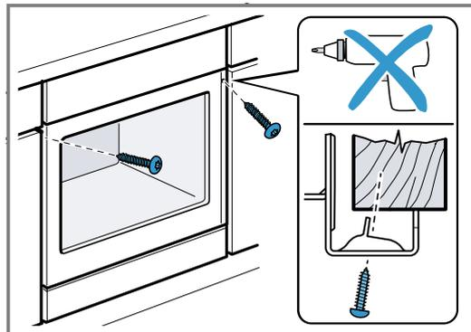
6. Refit the panels and screw them in place, first at the top and then at the bottom.
