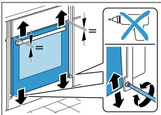
Turning the screws clockwise makes the gap smaller
