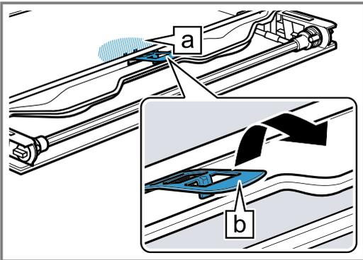
5. Lift the intermediate pane from below ① and remove it in the direction of the arrow ②.
