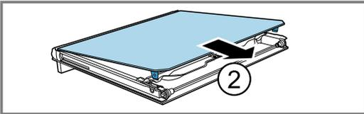
4. Push down on the intermediate pane in the area of [a], and carefully lift the retainer [b] until you are able to pull it out.
