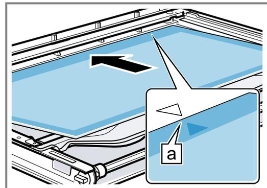
The arrow on the intermediate pane must line up with the arrow on the frame [a].
