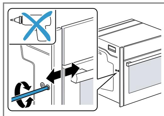
Turning the screws clockwise makes the gap larger
