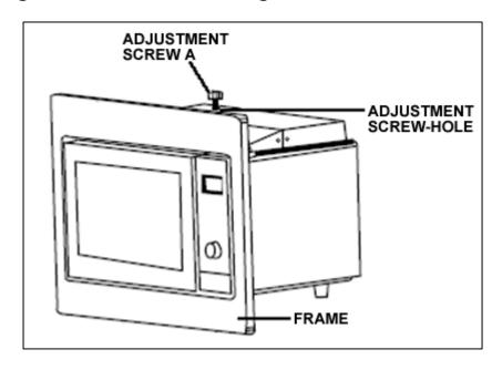
o Fit adjustment screw A into the adjustment screw-hole on the top of the microwave. Adjustment screw A should not be fully tightened at this stage.
