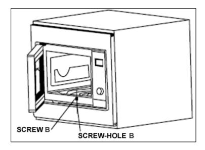
o Open the microwave door and locate screw-hole B. Use screw B to fix the microwave oven to the housing unit.
