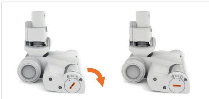
Refit the brushbar into the powered floorhead. Align the arrow on the brushbar cover so it points north, firmly push and twist clockwise to lock.
