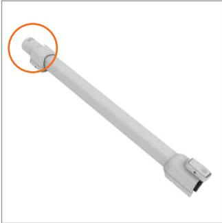
To test for a blockage in the reach wand, drop a small ball of paper into the wand. The paper will drop through if the wand is clear. Use a broom handle or similar blunt object to remove any blockage.
