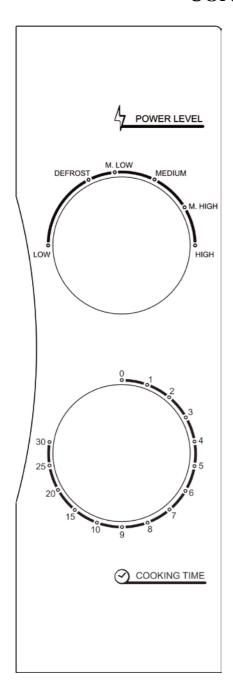
The control panel consists of two function operators. One is a time knob, and the other a power knob.
