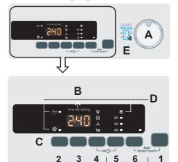
**A-Programme Selector -** Rotating the knob in both directions it's possible to select the desired drying program. To cancel the selections or switch off the dryer rotate the knob on OFF.
