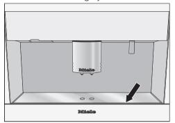
Replace the lid, and push the container back into place in the machine.
