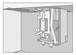
■ Press catch ① upwards slightly, grasp the dispensing unit by the handle and pull this forwards and off ②.
