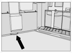
Remove the drip catcher and clean it in the dishwasher or by hand using hot water and a little washing-up liquid.
