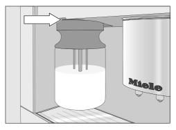
■ Push the milk flask fully back into the coffee machine.
