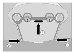
■ To remove, press and hold the sensor cover between the dispensers ①.
