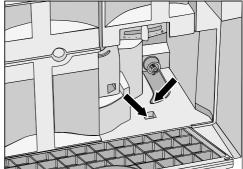
Carefully clean and dry the surface the water container sits on, taking special care to clean the recesses properly.
