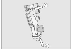
■ Reassemble the dispensing unit in the reverse order. Make sure that upper connecting piece ① clicks into position. Press dispensers ② firmly into position.
