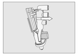
■ Hold the unit at the sides and pull it forwards to release it.
