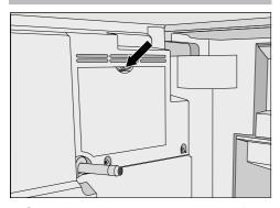
Open the maintenance panel on the back of the machine front.
