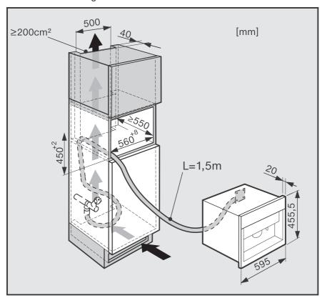
It can also be combined with other Miele built-in appliances. If the coffee machine is to be built in above another appliance, there must be a full-width, closed shelf between them (except when it is combined with a suitable Miele built-in plate or food warming drawer).
