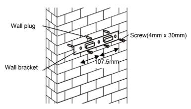
4. Leave up the cooker hood and hang onto the wall bracket hook.
