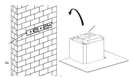
5. Fix the one-way-valve to the air outlet of the cooker hood. Then, attached the exhaust pipe onto the one-way-valve as shown below.
