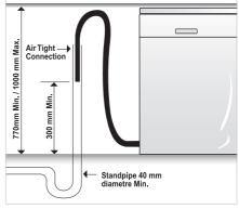
Fig. B: Drainage connection - stand pipe.
