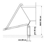
The free end should be positioned at a height of between **30 and 100 cm**, and should never be submerged in water.
