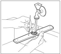
**4.** To install the spray arm back, insert the mounting element in the spray arm
