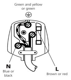
With the alternative plugs a 13A fuse must be fitted either in the plug or adaptor or in the main fuse box. If in doubt contact a qualified electrician.
