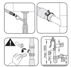
n Drain pipe must be connected to the sewage system and it should not be connected to any surface water.
