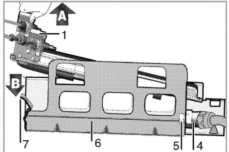
1. Unscrew 3 screws (2) to remove oven burner (1) and oven burner holder (7).
