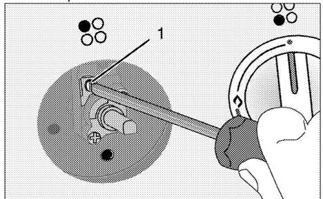
5. Set the flame length to 2 to 3 mm by means of the screw 1 on the oven tap. Turning in clockwise
