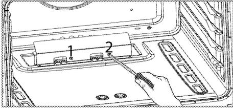
Unscrew 2 screws to remove burner protection sheet showing in the picture.
